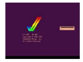
You can then insert either a Workbench disk or any other bootable disk such as a game into the floppy drive on the right-hand side of the Amiga (called DF0: - Disk Floppy Zero).
